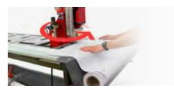
Unique 2 in 1 feature. One of the machines turns 180° and can be used as a standard eyelet press to finish the short sides of the banners.
