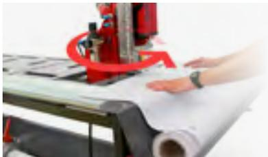
**Unique 2 in 1 feature.** One of the machines turns 180° and can be used as a standard eyelet press to finish the short sides of the banners.
