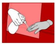
6. The next step is to heat the material gently, using a hot-air gun, to about 40°-50°C. The use of an AD laser temp will ensure your hitting this temperature range. It is advised to do small areas at a time.
