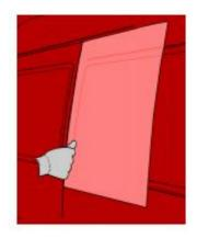
5. Now the application of the material in the corrugation can start. In order to be able to do so without forming wrinkles or creases, it is advised to wet the AD application glove, using a water/soap mixture.
