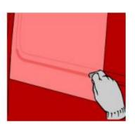
9. When all the deepest areas of the corrugation have been applied, the remaining part of the corrugation can be done. Again, make sure the material is heated to the required 40°-50°C, and work you way through the corrugation.
