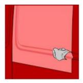
10. With all the edges properly applied, it is necessary to apply the material in the center of the corrugation. When doing this make sure that the air is not trapped, always leave an opening for the air to escape.
