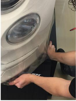
Conventional convex and compound shapes on car fronts are mostly suitable to be covered with all of the paint protection films in the Avery Dennison SPF series, but in some deeper corrugated shapes it may be necessary to make an incision in order to avoid any form of air/water entrapment in the deep recesses. This incision does not jeopardize the functionality or durability of the product.
